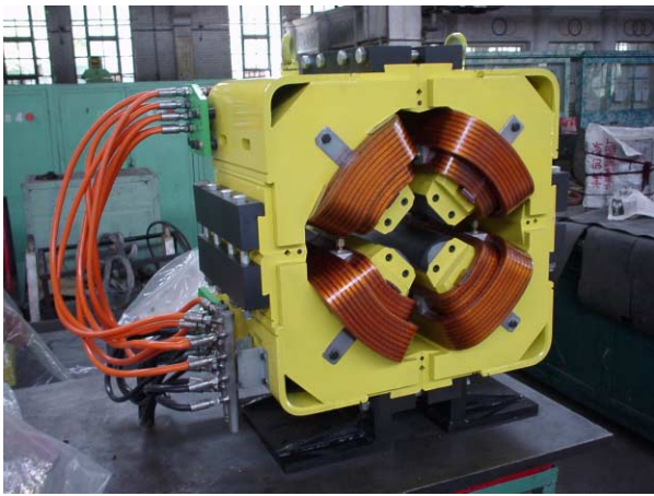
Fig. 16. Quadrupole prototype of CSR
