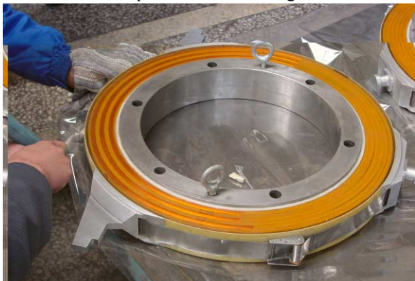
Fig. 17. Solenoid coil prototype of the CSR e-cooler
