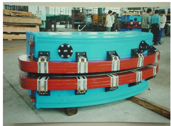
Fig. 15. 60^\circ C-type dipole prototype of CSR
