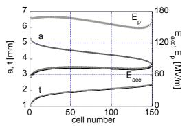
Figure: 1 Parameters of tested detuned structure. a if beam hole radius and t the disk thickness.  $E_{acc}$  is the average accelerating field in a structure without beam loading.  $E_{p}$  is the maximum surface field.
