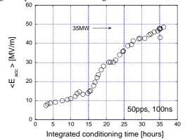
Figure: 7 Conditioning curve of 30cm-long structure.
