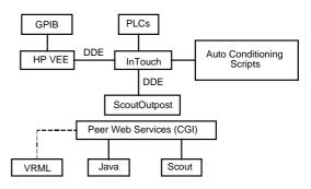
Figure: 3 Architecture of control and monitoring system for high field experiment of X-band structure.
