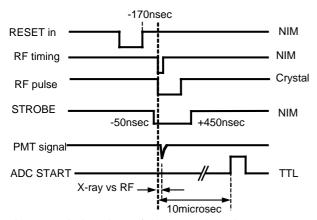
Figure: 5 Timing chart of the X-ray detection system.
