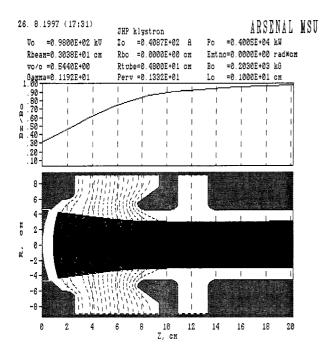
Figure 3: Modulation anode gun design of the klystron
