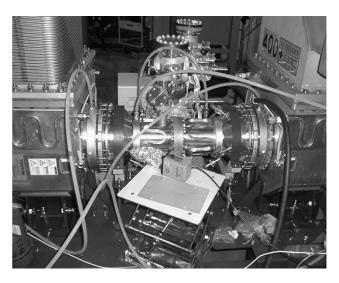
Figure 4: High power test of the co-axial window
