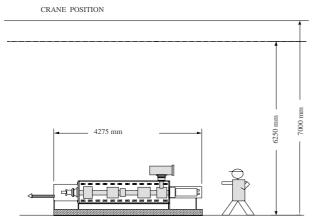
Figure 1: Horizontal mounting of the klystron
