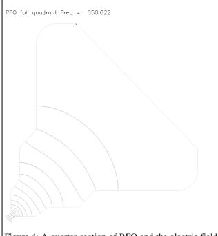
Figure 4: A quarter section of RFQ and the electric field calculated by SUPERFISH code.
