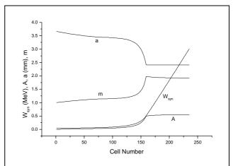
Figure 3: Key parameters such as the aperture (a), the vane modulation (m), the synchronous energy (W), and the acceleration strength (A) are shown along the cell.
