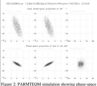
plots of the input beam and the beam at cell 240. The phase-space plots from left to right are: x-x', y-y', and phase-energy, where x'=dx/dz and y'=dy/dz.
