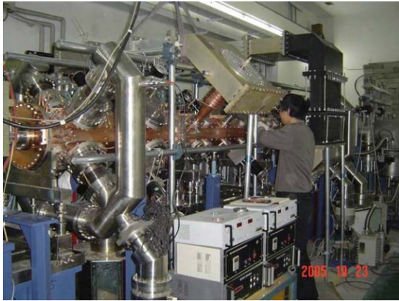
Figure 3: The 3.5 MeV, ADS RFQ under commissioning at IHEP, China. The first proton beam was injected from the ECR ion source and successfully extracted with a transmission efficiency of about 92% on a proton beam of 43 mA peak current. The beam duty factor reached 6% with beam of 1.2 ms pulse length running at 50 Hz.
