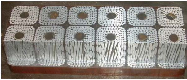
Figure 6: One of the first prototypes of the J-PARC type stranded magnet coil fabricated by a vendor in China.
