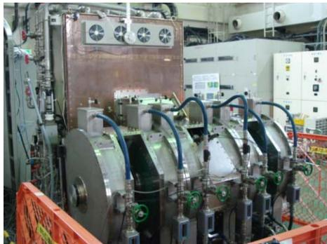
Figure 4: The cut-core loaded cavities under long-term continuous operation with nominal voltage of 15 kV/gap and 60 % duty.
