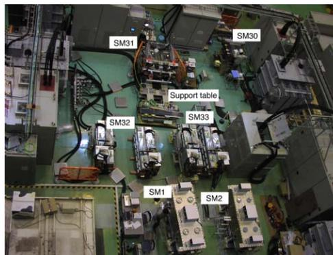
Figure 3: Fast-extraction septum magnets. SM31 is under testing.
