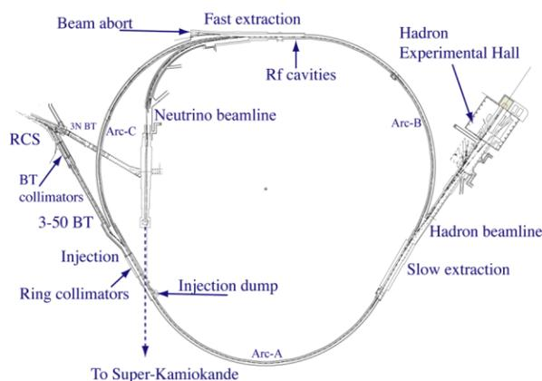
Figure 1: Plan view of MR and experimental facilities.
