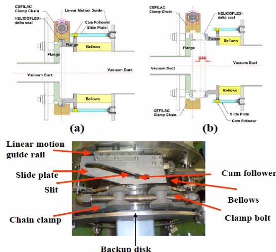
Figure 3: Semi-remote handling vacuum flange(a) Loosen the chain clamp, (b) compress the bellows
