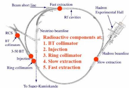
Figure 1: Location of radioactive components
