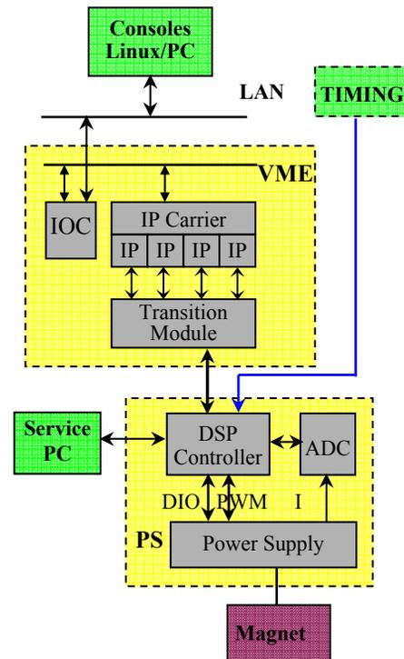
Figure 1: The PS control system architecture
