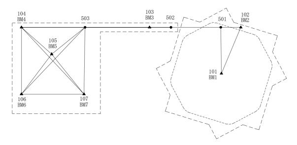
Fig.5 The Survey network for 1st order reference marks
