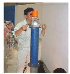
Fig.7 Centering by optical plummet on the auxiliary pillar
