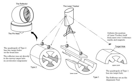
Fig.15 Scheme of alignment by the laser tracker
