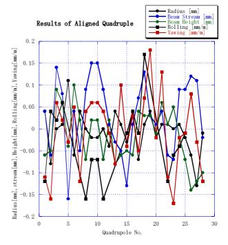
Fig.17 Results of the alignment for quadrupoles
