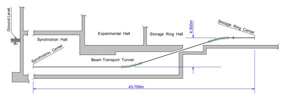
Fig.2 Profile of the acelerator complex of the SPS
