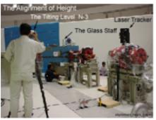
Fig.13 The alignment for the dipole
