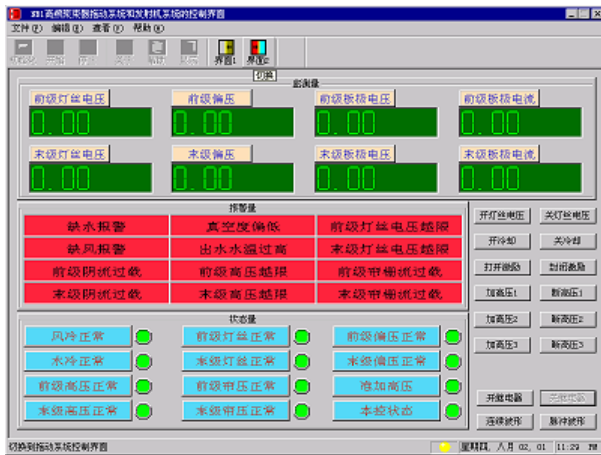
Fig.2 The interface of the computer control of RF Emitter
