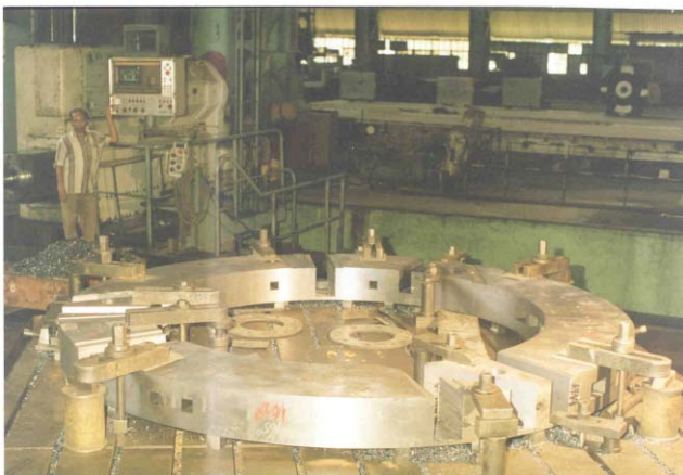
Figure 4 : Machining of the central return path ring for the main magnet frame.
