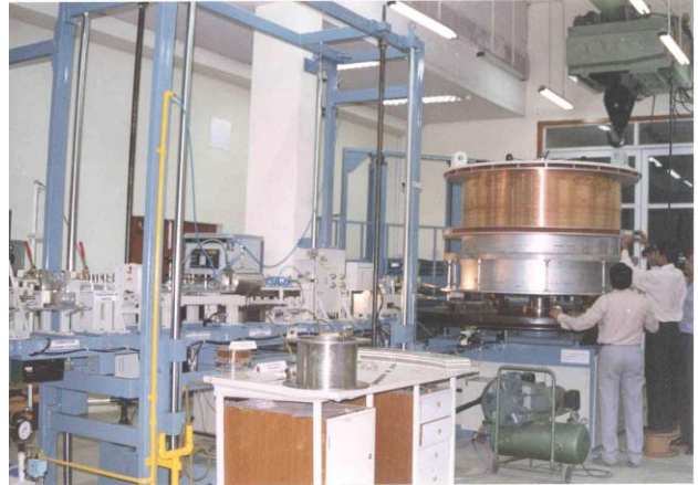
Figure 5 : Superconducting coil winding setup at VECC.
