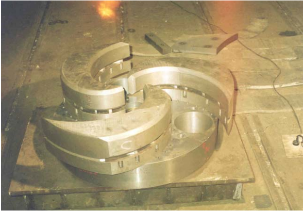
Figure 3 : Pole tips assembled on the pole base for inspection at the fabrication site.
