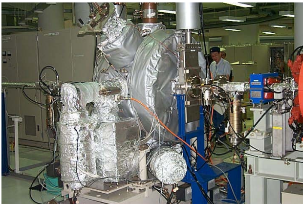
Figure 3: The RF cavity installed in the storage ring during baking
