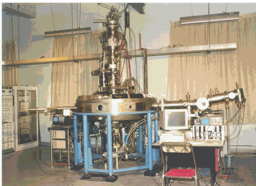
Figure 4: Shanghai Mini-Cyclotron-based Accelerator
