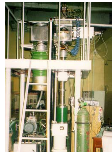
Figure 7: The test stand of the H- ion source and axial injection line.
