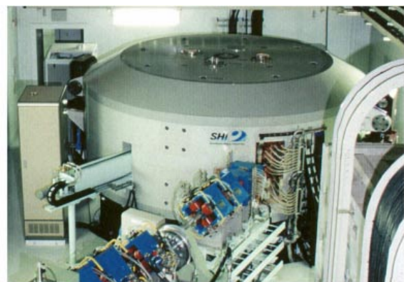
Fig. 7: A 235 MeV fixed energy AVF cyclotron for proton therapy at National Cancer Center Hospital East.
