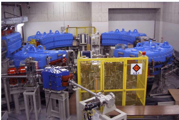
Fig. 11: A synchrotron ring for Shizuoka Cancer Center under final beam tests at an accelerator maker.
