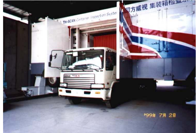
Figure 13: relocatable type inspection system
