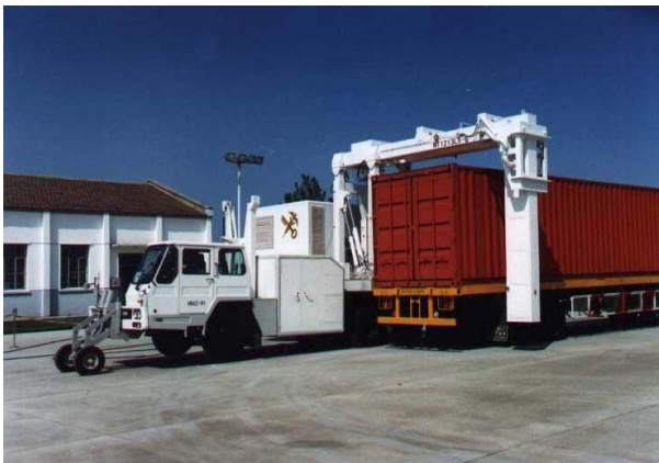
Figure 12: mobile container inspection system
