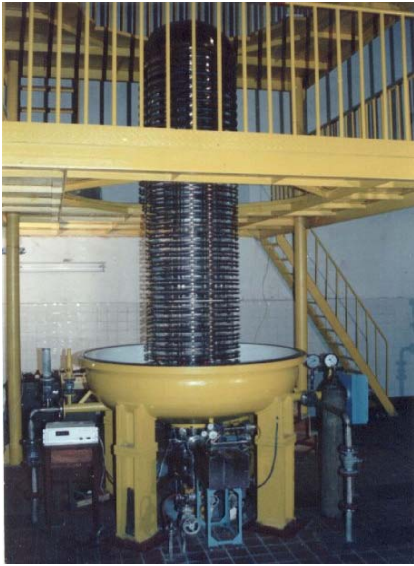
Figure 4: 3.0MeV Dynamitron-type machine made by SINR.
