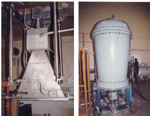
Figure 9: The 800~1200 KV 80 mA accelerator at LIMPR
