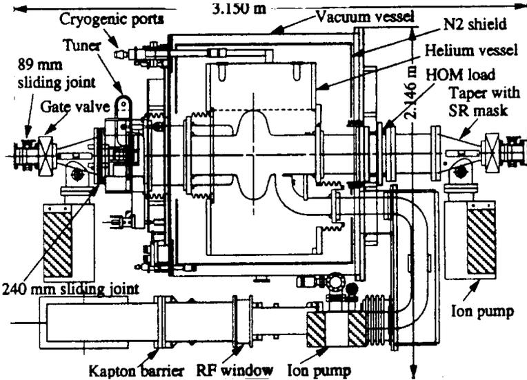
Fig. 6: SC cavity-cryostat system for CESR-III [12].
