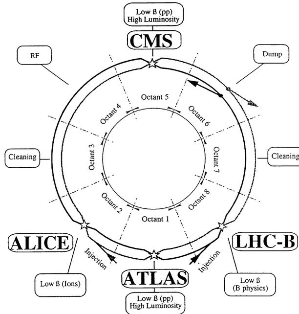
Fig. 4: Schematic layout of LHC [7].
