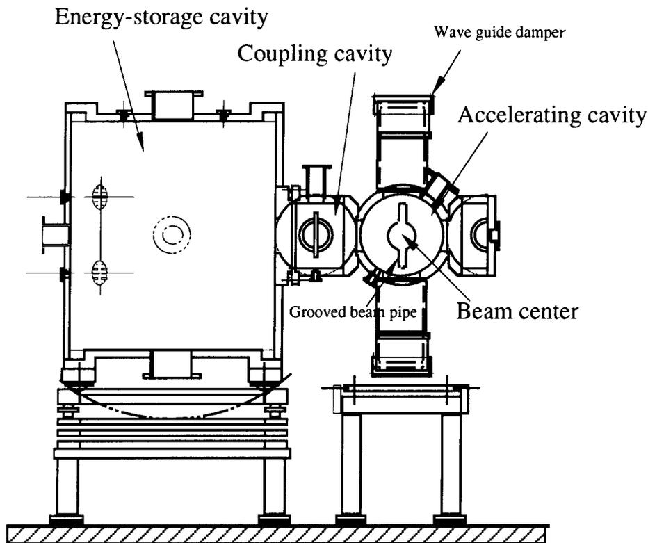
Fig. 7: The ARES NC cavity [15].
