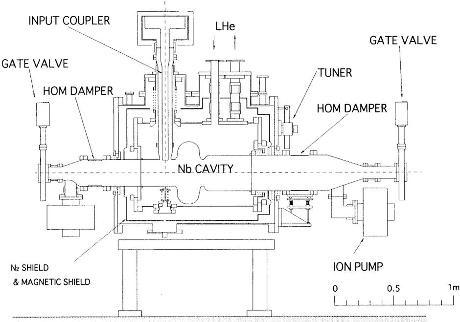
Fig. 5: SC cavity-cryostat system for KEKB [10].
