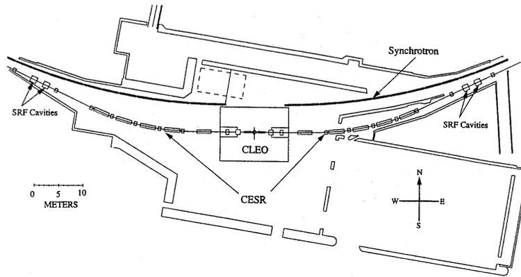
Fig. 2: Schematic layout of CESR phase III near the interaction region [12].
