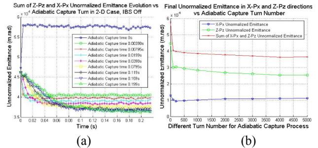
Figure 3: (a) The sum of X-Px and Z-Pz un-normalized emittance evolution vs. different adiabatic capture time in 2-D case (b) Final un-normalized emittance in X-Px and Z-Pz directions vs. adiabatic capture turn number.
