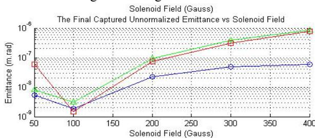
Figure 5: Result combination of cooling result vs. different solenoid field.
