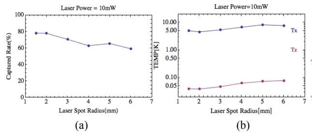
Figure 4: Laser profile parameter optimization of certain power of laser in 2-D laser cooling. (a) Capture rate of laser cooling using different vs. laser spot radius, (b) The final temperature of captured particles vs. laser spot radius, IBS on, number of particles simulated is 300.
