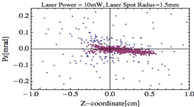
Figure 2: A typical phase-space plot after laser cooling. The magenta dots represent captured particles while blue dots shows hot beam corona.
