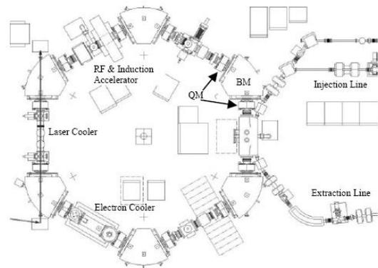
Figure 1: Layout of the ion storage ring [9].
