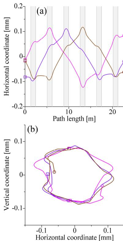
Figure 4: (a) Single-particle orbits of the beam in Fig. 3 while the beam circulates the storage ring once. The horizontal orbits of three ions arbitrarily picked out from the ordered beam are shown. The six gray shaded areas indicate the bending-magnet sections. (b) The trajectories of the three ions in the cross-sectional view are shown. In both panels, the square and circle symbols represent the initial and final coordinates of the ions during one turn, respectively.
