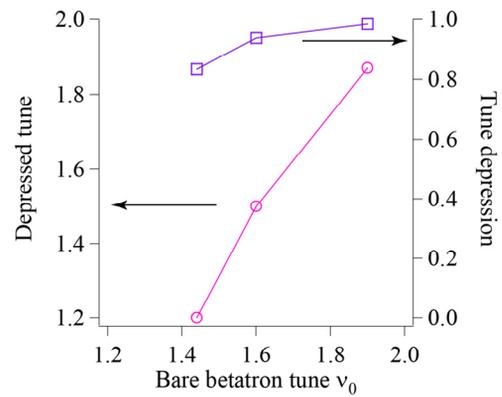
Figure 5: Depressed tune and the tune depression of 3D ordered beams formed at different operating points.
