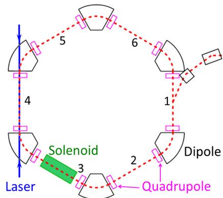
Figure 1: Schematic drawing of S-LSR. The circumference of the ring is 22.56 m. Six bending dipole and 12 quadrupole magnets have been excited so that the six-fold lattice superperiodicity can be realized. Numbers (1 to 6) in the figure express the number of straight sections for convenience. Two cooling lasers are injected along the fourth straight section. A solenoid magnet, installed in the middle of the third coupling section, is excited for horizontal-vertical coupling.
