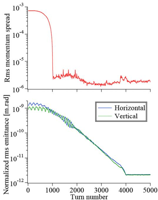
Figure 2: Time evolution of the longitudinal momentum spread and transverse emittance of the 40-keV  $^{24}\text{Mg}^+$  ion beam during laser cooling. The bare betatron tune  $\nu_0$  is 1.44. The line density of the beam is  $2.4 \times 10^4 \text{ m}^{-1}$ . The laser detuning is scanned in 1000 turns. The horizontal displacement and final detuning of the lasers are 3 mm and -81 MHz, respectively.
