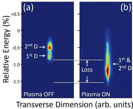
Figure 1: Images of the bunch train with two drive bunches (no witness bunch) dispersed in energy in the vertical direction, with (a) the plasma off, and (b) a plasma density of  $\approx 8 \times 10^{15} \text{ cm}^{-3}$ .
