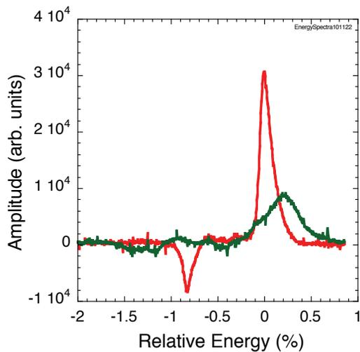
Figure 3: Energy spectra obtained by subtracting the plasma off images (1(a) and 2(a), plasma off, red line) from the plasma on images (1(b) and 2(b), plasma on, green line). The witness bunch charge distribution is centered around the zero relative energy. The negative peak near relative energy  $-0.8\%$  on the plasma off case corresponds to a slightly different charge distribution between the two images (1(b) and 2(b)). Plasma density of  $\approx 8 \times 10^{15} \text{ cm}^{-3}$ .
