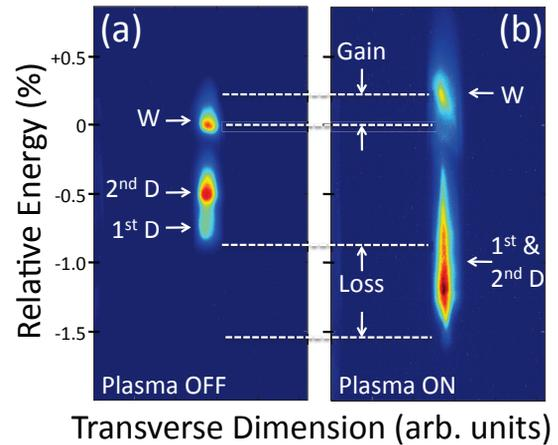
Figure 2: Images of the bunch train with two drive bunches and the witness bunch dispersed in energy in the vertical direction, with (a) the plasma off, and (b) a plasma density of  $\approx 8 \times 10^{15} \text{ cm}^{-3}$ .
