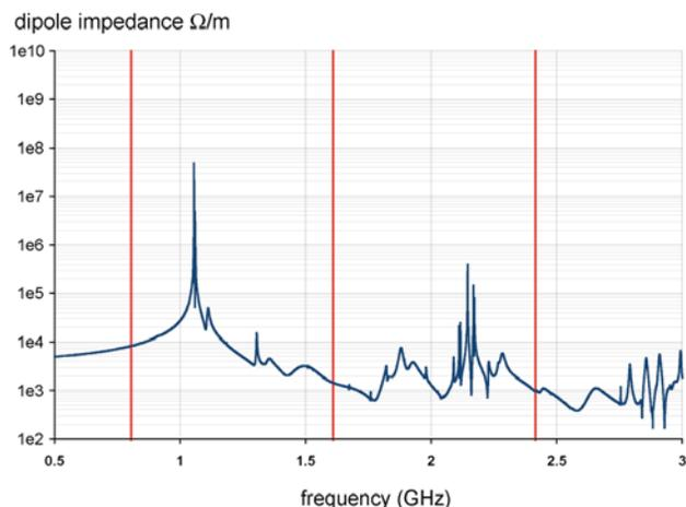
Figure 6: High-current  $\beta=0.65$  cavity dipole spectrum.
