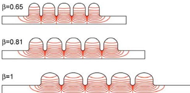
Figure 2: Cavity profiles and fields from Superfish.
