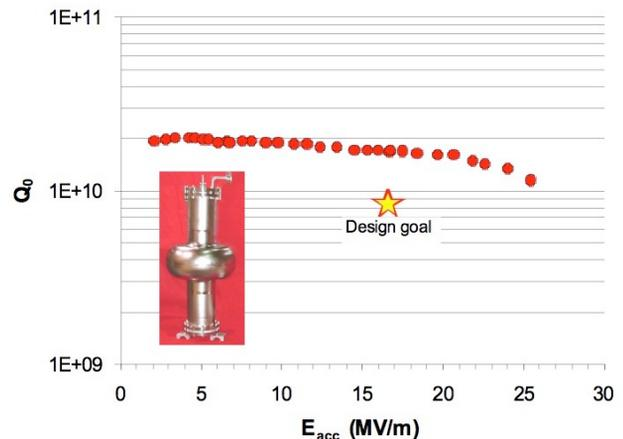
Figure 4: Test result of single cell 750 MHz  $\beta=1$  cavity after BCP processing.
