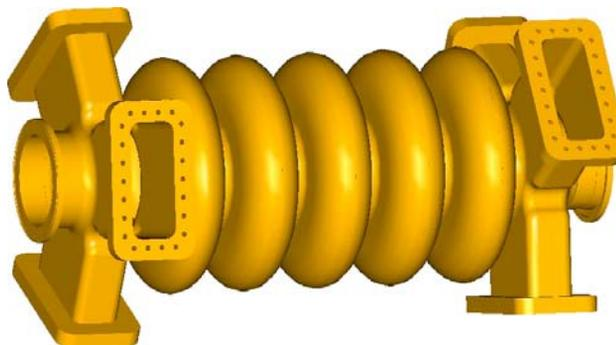
Figure 1: Cavity with rounded high-current  $\beta=0.85$  cells, waveguide HOM dampers and fundamental power coupler.
