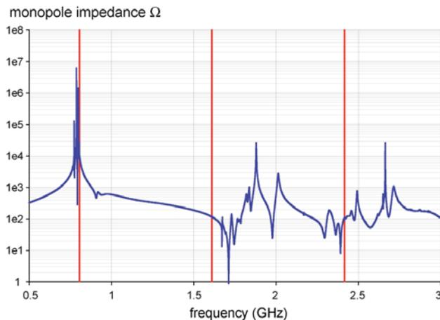
Figure 5: High-current  $\beta=0.65$  cavity monopole spectrum.
