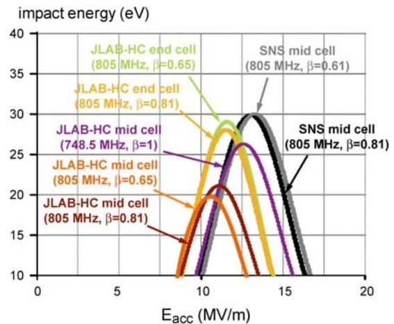
Figure 3: Electron impact energy on stable resonant trajectories calculated by Fishpact.
