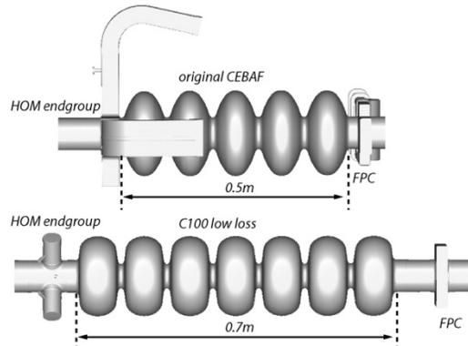
Figure 2: 1497 MHz original CEBAF 5-cell cavity in comparison to the low loss 7-cell upgrade style cavity.
