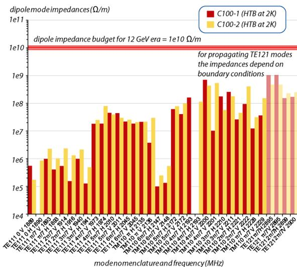
Figure 5: Dipole mode impedances in C100-1 and C100-2 respectively as measured in the HTB at 2K.
