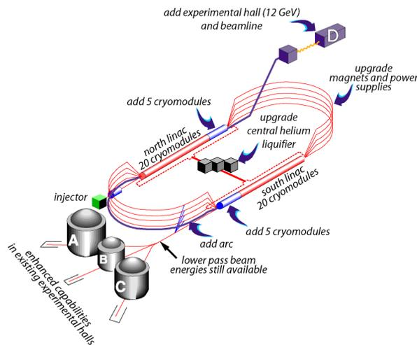
Figure 1: Layout of CEBAF indicating the planned upgrades to provide up to 12 GeV beam energy with 5½ recirculating passes using CW SRF linac technology.
