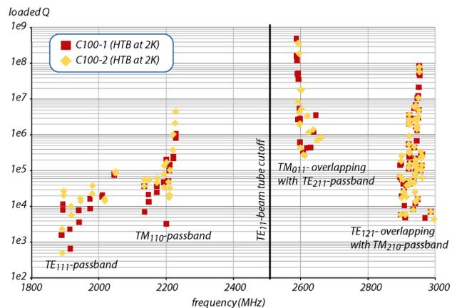
Figure 4: Loaded HOM Qs measured in the HTB at 2K.
