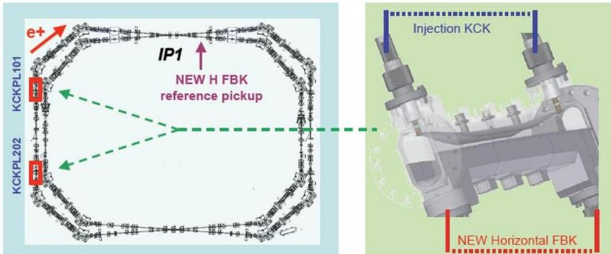
Figure 2: DAFNE main rings layout with new horizontal pickup and hybrid kicker positions.
