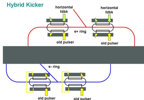
Figure 1: Hybrid kickers for injection and feedback.
