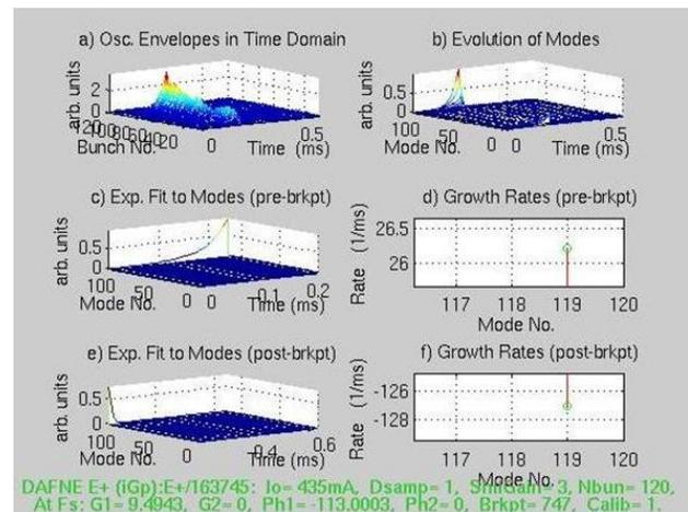
Figure 3: Single feedback damping rate [ $128 \text{ ms}^{-1}$ ].
