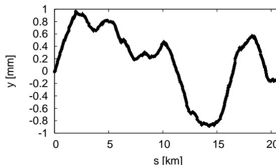
Figure 3: An example of the misalignment of the main linac elements due to the wire reference system.
