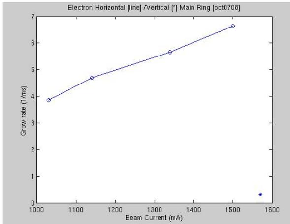
Figure 3: DAFNE e- horizontal instability grow rates versus beam current [October 7, 2008].
