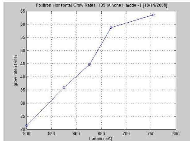
Figure 2: DAFNE e+ horizontal instability grow rate versus beam current [10/14/2009].
