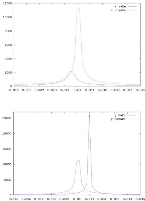
Figure 3: Results of simulation of wakefield effects in rectangular geometry. Top plot shows an FFT of the x position of the beam for the cases of a wakefield present, and no wakefield present. The bottom plot is similar, except it is y-plane data.
