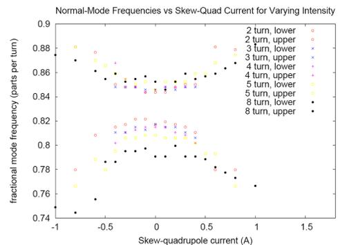
Figure 1: Measured mode frequencies vs. skew quadrupole circuit current at varying intensities. At each intensity there are two curves (plotted with the same symbol) which correspond to the dependence of upper and lower mode frequencies on the skew quadrupole current. The separation of the upper and lower curves is a measurement of the minimum coupling.
