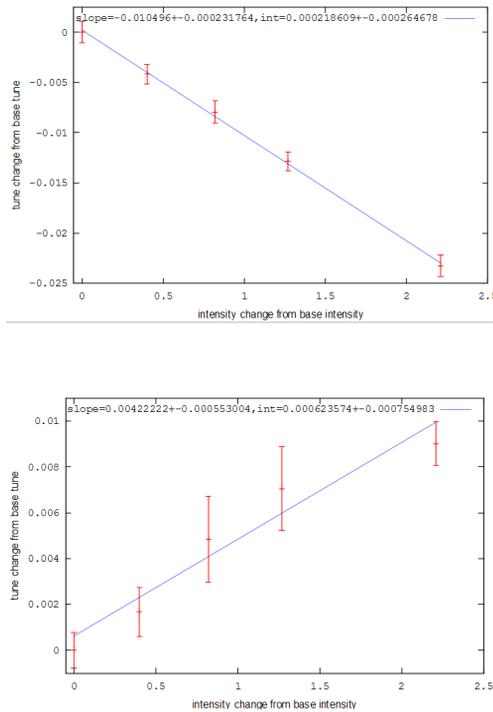
Figure 2: Mode frequency vs. beam intensity. The x-axis is the beam intensity in units of  $10^{12}$  protons, and the y-axis is the change in tune (mode frequency) with respect to the tune (mode frequency) at the low intensity data point.
