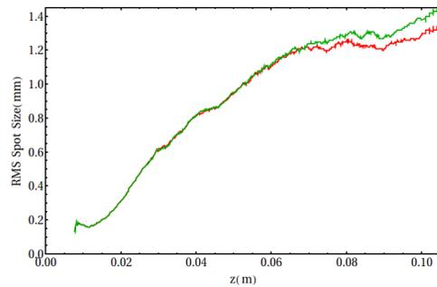
Figure 6: Plot showing the RMS spot size of the electron beam along the compact linac calculated using ASTRA. The red line shows the spot size for the ideal cavity and the green line shows the spot size for the actual cavity.
