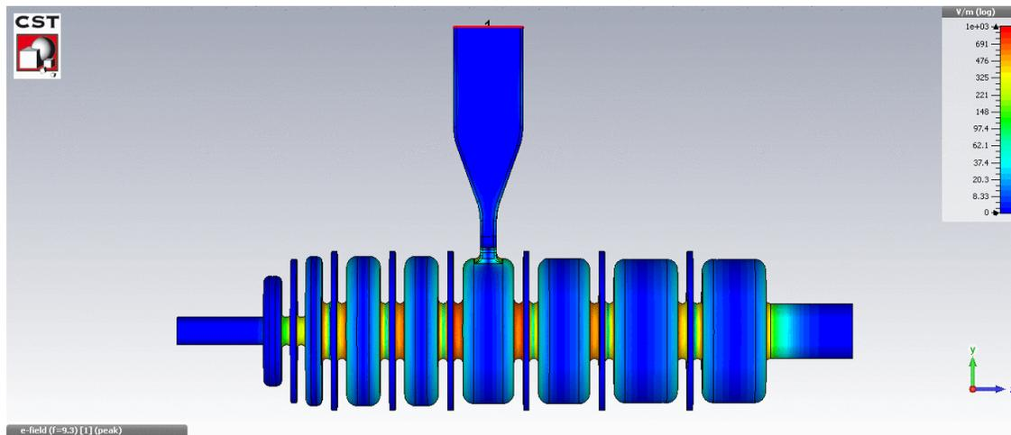
Figure 2: Final RF design of x band linac simulated in CST Microwave Studio. Image is of the electric field distribution in the final cavity.
