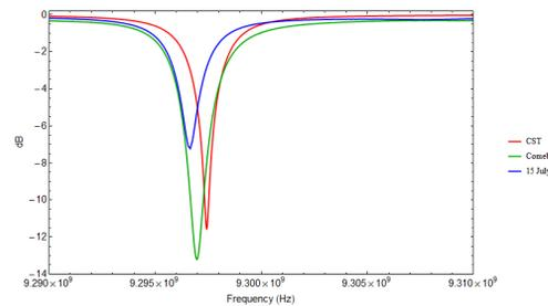
Figure 3: Magnitude of S11 for the x band cavity. The expected S11 measurement calculated in CST is shown in red, the S11 measurement performed by the manufacturer is shown in green and the S11 measurement performed on receipt of the cavity is shown in blue.
