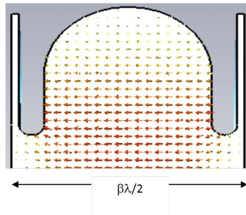
Figure 1: A single cell in a bi-periodic standing wave cavity.
