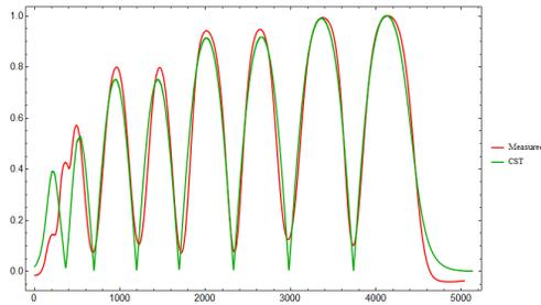
Figure 4: Field flatness plot showing how the electric field varies along the axis of the cavity. The red line shows the measured field flatness and the green line the expected field flatness.
