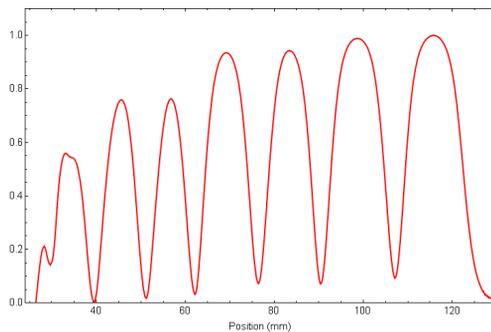
Figure 5: Field flatness plot showing how the electric field varies along the axis of the cavity after initial tuning.
