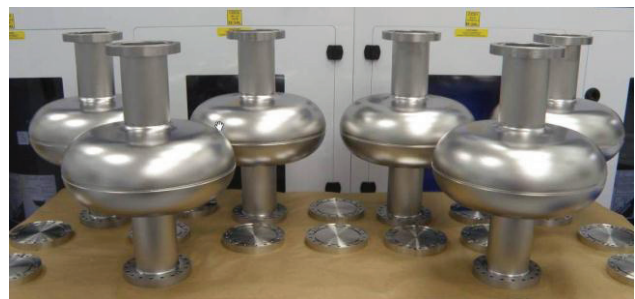
Figure 8: Six AES cavities complete in-house.
