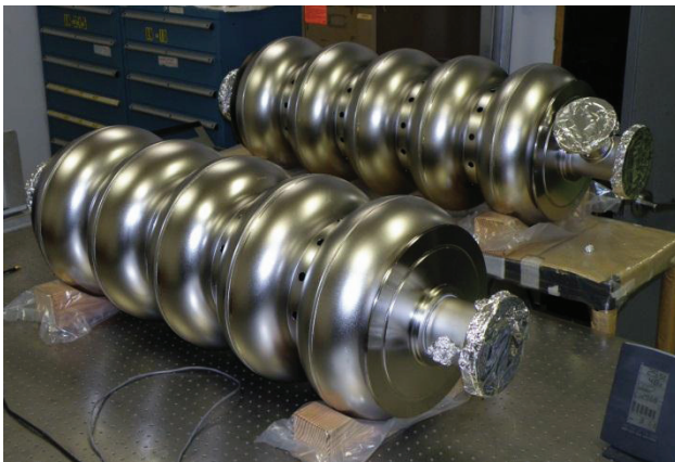
Figure 10: Two AES 5-cells cavities
