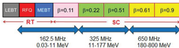
Figure 1: The PIP-II Linac Layout.
