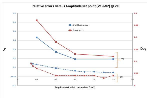
Figure 4: Measured performances on a Spoke cavity at 2K of the two prototype DLLRF systems (rms values).
