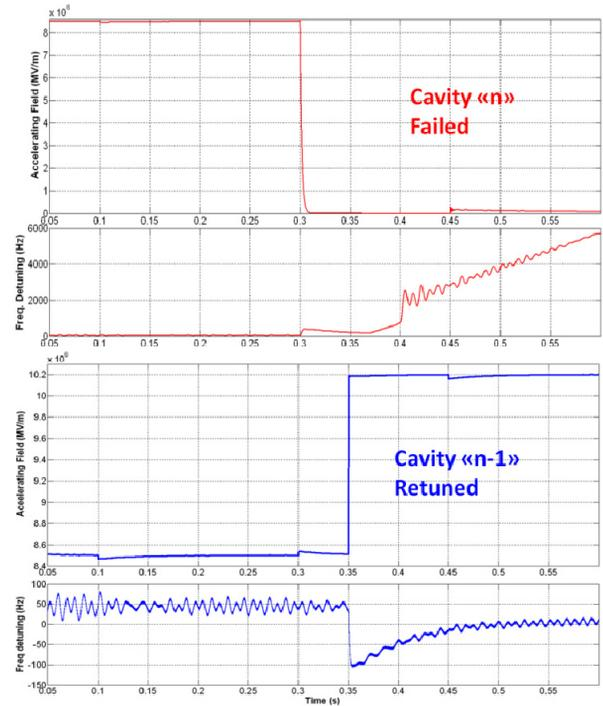
Figure 2: Simulation results for the update of two adjacent cavities during a “fast fault-recovery” scenario.
