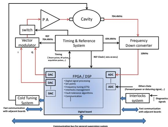
Figure 3: ADS-type LLRF system general scheme.
