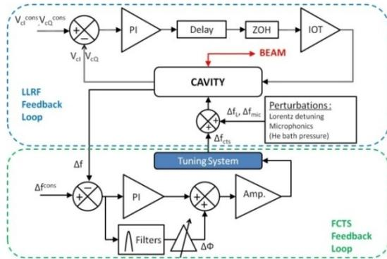
Figure 1: Bloc diagram describing all the modeled elements of the LLRF and tuning System feedback loops.
