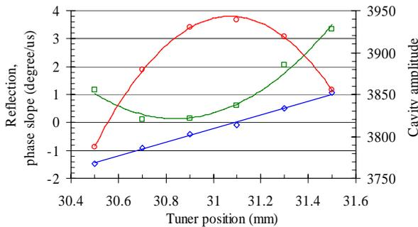
Figure 6: Cavity amplitude (red curve), reflection from cavity (green curve), and cavity phase slope during field decay (blue curve), as function of tuner position for BUN2.
