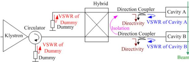
Figure 3: Setup of RF systems at the SDTLs of the J-PARC LINAC.
