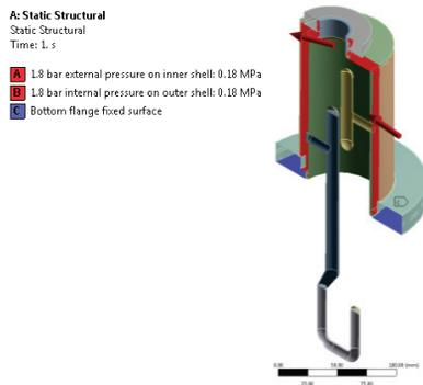
Figure 5: HOM coupler assembly – boundary conditions.
