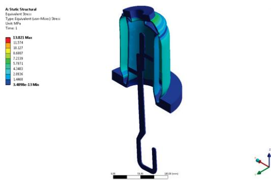
Figure 6: HOM coupler assembly – stresses.
