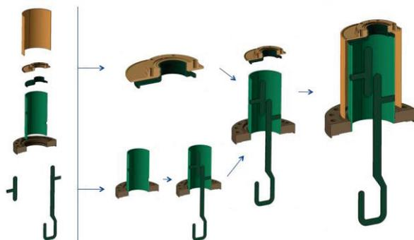
Figure 7: Assembly sequence.
