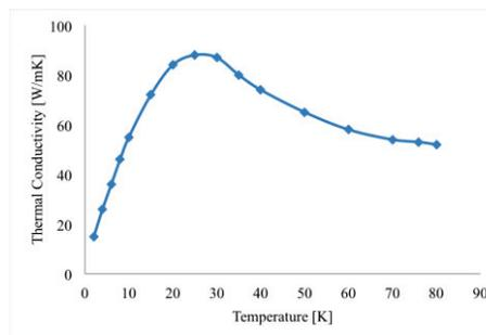
Figure 2: Temperature dependent thermal conductivity of niobium.
