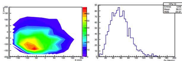
Figure 4: The negative muon flux at the 36° curved transport solenoid (left) and The negative muon momentum distribution at the 36° curved transport solenoid (right).
