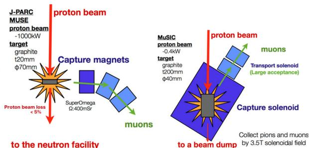
Figure 2: A conventional muon beam facility (left) and the pion capture system of MuSIC (right)..
