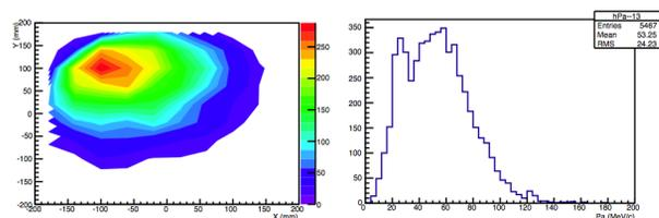
Figure 3: The positive muon flux at the 36° curved transport solenoid (left), and the positive muon momentum distribution at the 36° curved transport solenoid (right).
