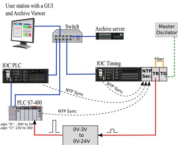
Figure 1: Timing correlation prototype.
