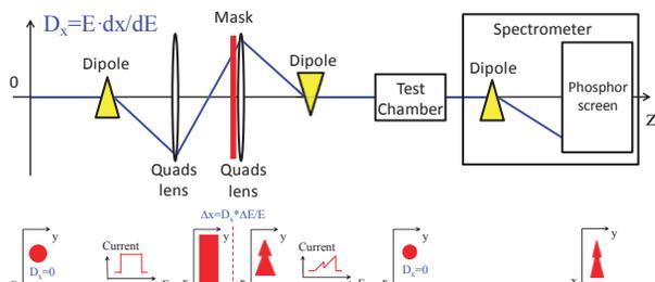
Figure 3: Schematic of beam shaping at ATF.
