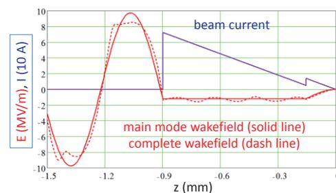
Figure 2: DT current and its wakefield in the tube chosen for the experiment:  $a=550 \mu\text{m}$ ,  $b=400 \mu\text{m}$ ,  $\epsilon=3.8$ .
