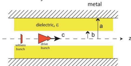
Figure 1: Schematic of the DWA.
