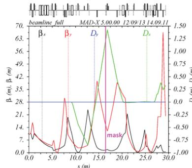
Figure 4: Twiss parameters as modeled in MAD-X vs the beam propagation distance with the mask location marked.
