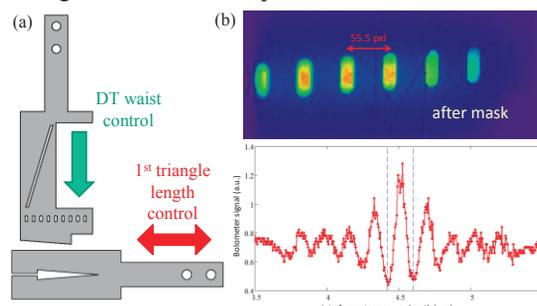
Figure 5: Adjustable beam mask (a). Longitudinal size calibration using coherent transition radiation interferometry (b).
