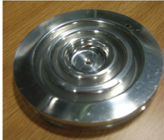
Figure 1: A two-choked 8 GHz Al test cavity.
