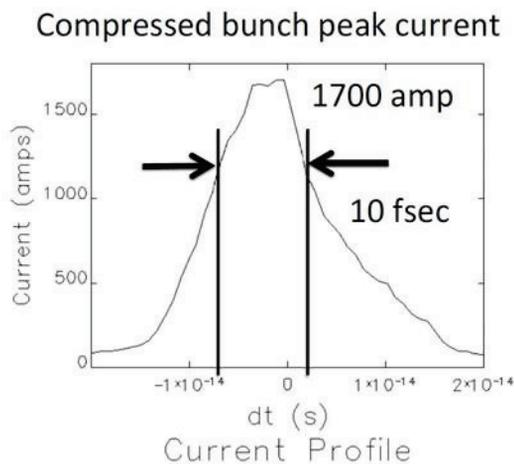
Figure 2: Compressed bunch profile (modelled using ELEGANT [11]).
