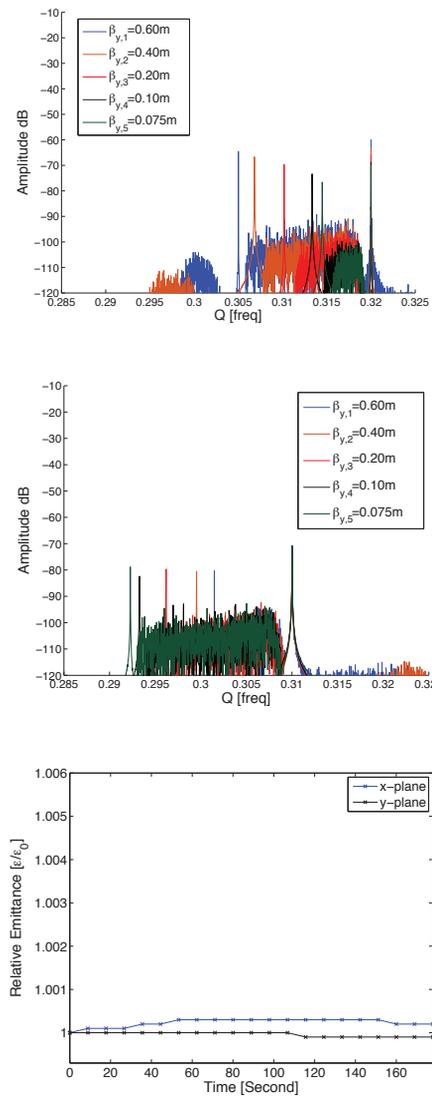
Figure 2: The top plot shows the dipole modes in the vertical plane during the levelling steps for the flat beam profile. The middle plot; shows the dipole modes along the horizontal plane during the levelling steps and the bottom plot; shows the mean emittance throughout the levelling process with the vertical plane given by the blue line and the horizontal plane is given by the black line.
