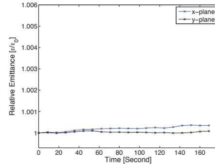
Figure 1: Figure top; shows the dipole modes in the vertical plane during the levelling steps. Figure middle; shows the dipole modes along the horizontal plane during the levelling steps. Figure bottom; shows the mean emittance throughout the levelling process. The slight emittance growth in each plane can be attributed to numerical noise with the vertical plane given by the blue line and the horizontal plane is given by the black line.
