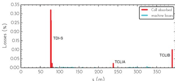
Figure 3: Simulated loss map of Beam 1 in case of MKI kick error of ~11% (grazing impact on TDI in case of ideal machine) considering the machine configuration where the highest losses were seen on the TCLIB.
