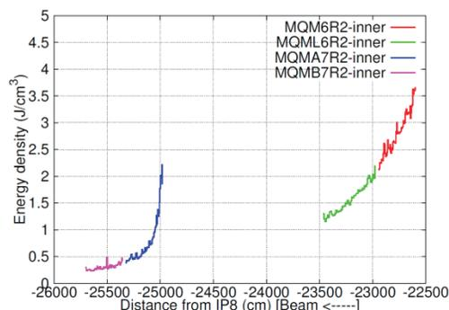
Figure 5: Longitudinal peak energy density in the inner coils of the quadrupoles Q6 and Q7.
