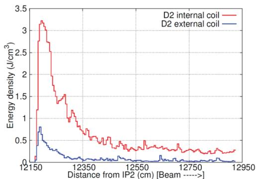
Figure 4: Longitudinal peak energy density in D2 coils.
