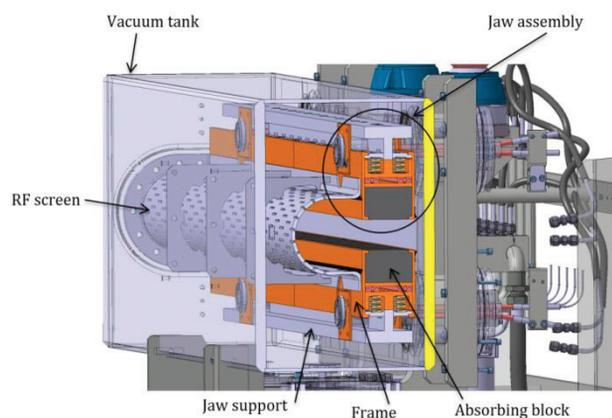
Figure 1: Preliminary design of one TDIS module.
