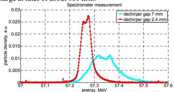
Figure 6: Energy spectra of the beam passing through a dechirper with gap sizes: 7 and 2.4 mm. The energy spread reduction is observed.
