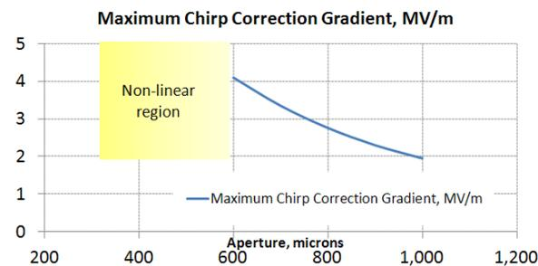
Figure 4: Chirp correction gradient as a function of the aperture size for a tunable dechirper consisting of 1 mm thick alumina plates.
