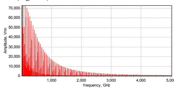
Figure 2: Spectrum of modes excited by the  $\sigma_z = 10$  micron gaussian beam (equivalent to the rising edge of the quasi-rectangular beam) inside the 1 mm thick alumina plates, 600 micron gap structure.
