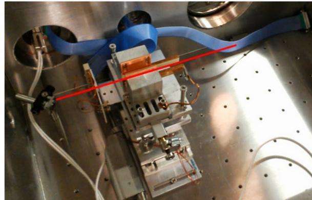
Figure 5: Chirp corrector in the ATF beamline. The beam path is marked with a red line.
