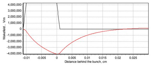
Figure 3: Almost linear decelerating field generated inside the quasi-rectangular beam passing through the 1 mm thick alumina plates, 600 micron gap structure.
