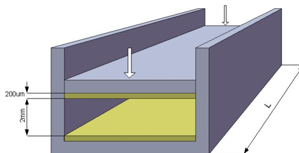
Figure 1: Conceptual design of a tunable dielectric loaded rectangular chirp corrector.
