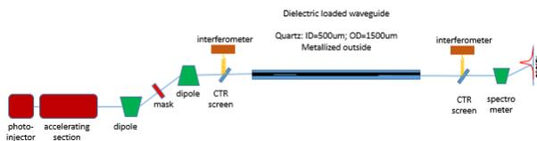
Figure 2: Experiment setup at ATF beamline.
