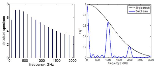
Figure 1: Left: Cherenkov spectrum of the multi-mode wakefield structure. Right: Formfactor of single bunch and bunch train.
