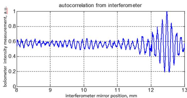
Figure 4: Interferometer measurement of the Cherenkov radiation mixed with coherent transition radiation: bolometer signal intensity as a function of interferometer mirror position.
