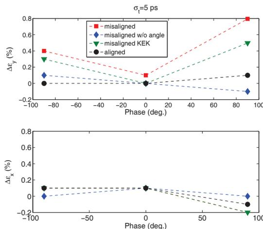
Figure 7: Relative emittance growth in both vertical planes versus  $\phi_{acc}$  for the different scenarios studied for the first booster cavity behind the SRF photo-injector in reference to the bare cavity using the PIC code.
