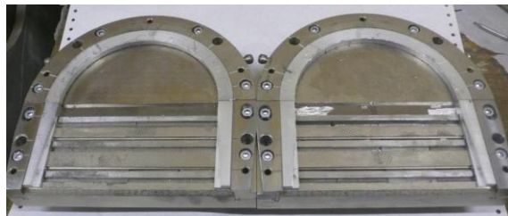
Figure 3: Two halves of the end magnet.
