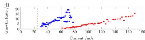
Figure 7: Measurement of the growth rates of the horizontal instabilities at various beam currents.
