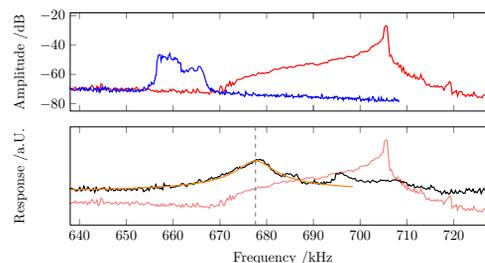
Figure 3: Beam spectrum measurement of the lower horizontal betatron sideband, measured at 100 mA.
