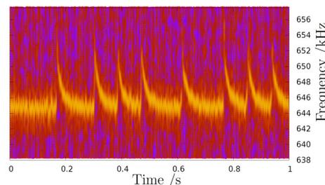
Figure 4: Dynamic behavior of the tune of the horizontal instabilities at 94 mA.
