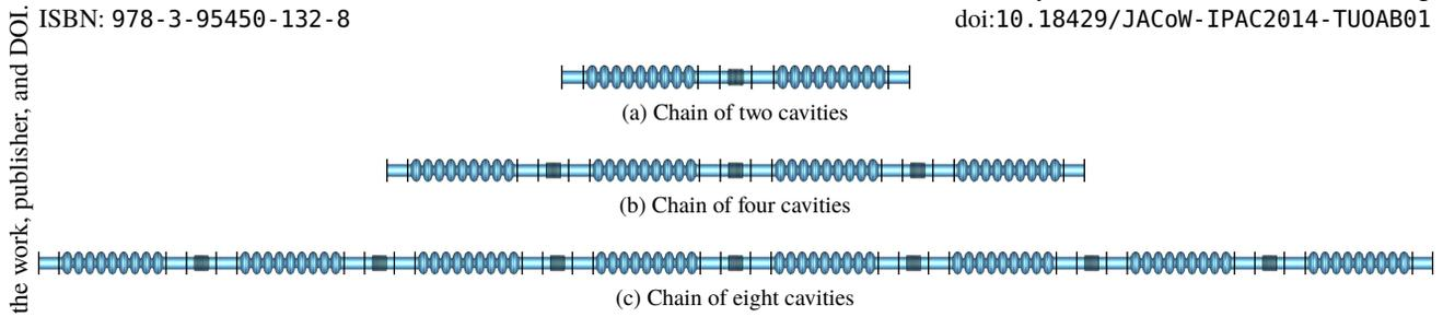
Figure 1: Investigated cavity chains with bellows in between. Structure (a) is solely used for validation purposes, (b) models the third harmonic cavity chain in FLASH, and (c) reflects the chain for the European X-FEL respectively.
