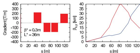
Figure 4: “Pushed” IR optics with  $\beta^* = 0.3 \text{ m}$  and a free length  $l^*$  of 36 m ( $l^* = 23 \text{ m}$  at the LHC) [15].
