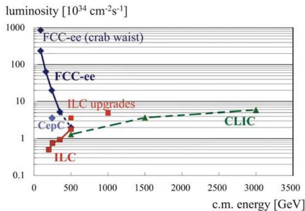
Figure 5: Projected total electron-positron luminosities vs. c.m. energy for various proposed colliders.
