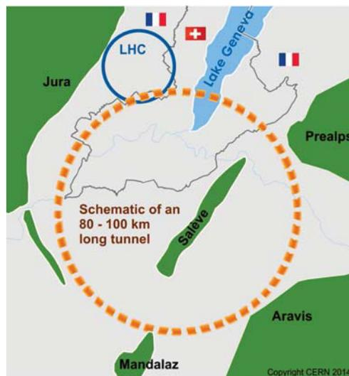
Figure 1: Schematic of a 100-km tunnel for a highest-energy circular collider in the Lake Geneva basin.
