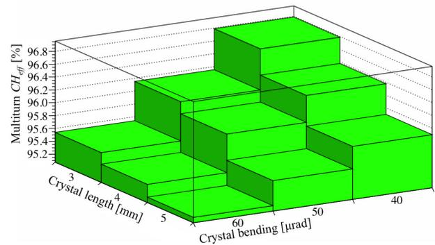
Figure 3: Multiturn channeling efficiency ( $CH_{eff}$ ) for different combinations of crystal bendings and lengths probed.
