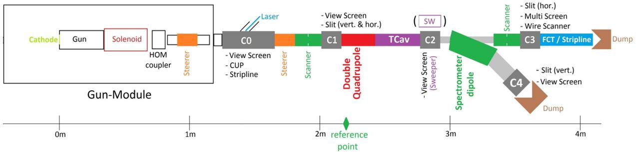
Figure 1: Schematic view of GunLab.
