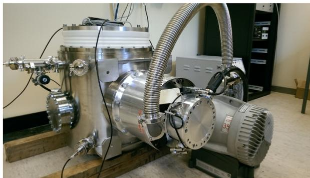
Figure 2: VESPA vacuum vessel undergoing testing.
