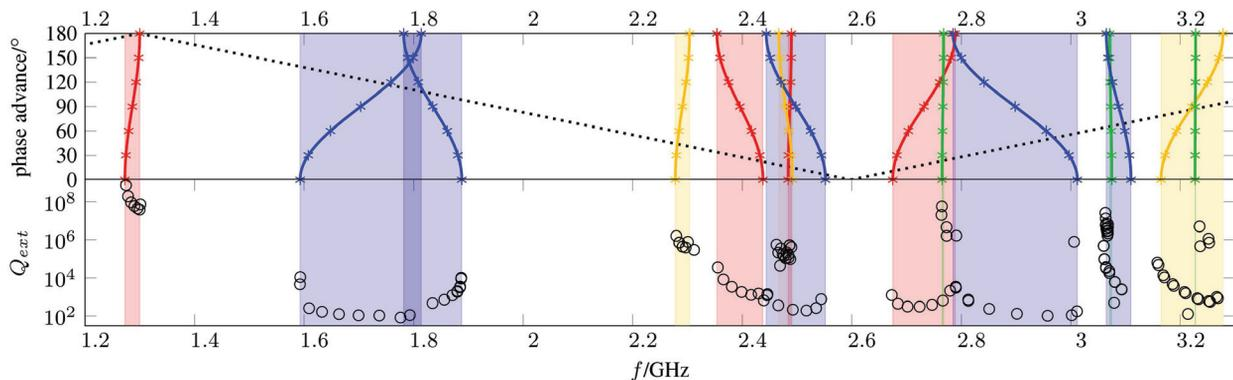
Figure 3: Band diagram for the 7-cell cavity (top) and a set of  $Q_{ext}$  factors for the design candidate nr. 5. The indicated bands are colored according to the type of the mode, that is, monopoles (red), dipoles (blue), quadrupoles (orange) and sextupoles (green). The external quality factors (black circles) were automatically obtained using the vector fitting and TPE procedure.
