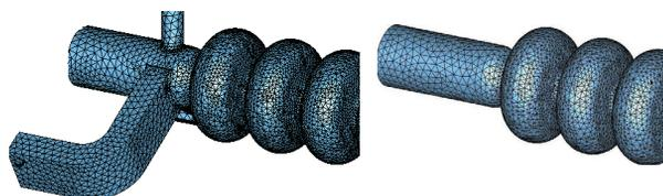
Figure 1: Comparison of the SRF cavity with (left) and without (right) the coaxial power coupler and the waveguide HOMs couplers.
