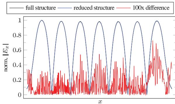
Figure 2: Comparison of the axial electric field strength for the full structure and the reduced structure without the coaxial and the waveguide couplers. The maximum of difference of these two profiles does not exceed 0.75%, indicating none or very small influence of the HOMs waveguide couplers on the field flatness.
