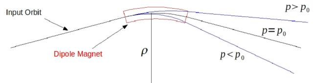
Figure 1: Dispersion induced by bending magnet. Electrons exit dipole separated from design orbit according to differing momenta.
