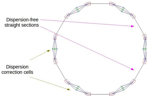
Figure 3: Chasman-Green DBA lattice for traditional ring configuration.
