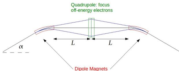
Figure 2: Dispersion correction by quadrupole magnet. Electrons of all momenta exit second dipole on design orbit.
