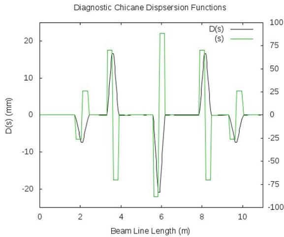
Figure 5: TRANSPORT simulation results of Diagnostic Chicane dispersion function and derivative.
