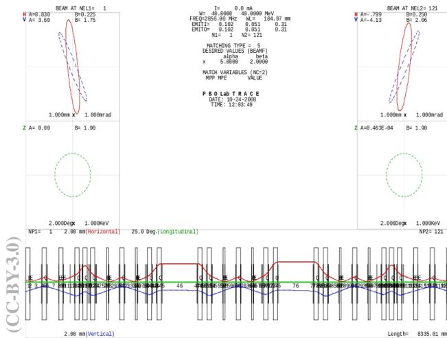
Figure 6: Examples of quadrupole triplet and doublet pair focusing schemes in Diagnostic Chicane, red trace is the horizontal envelope; the blue trace is the vertical envelope.
