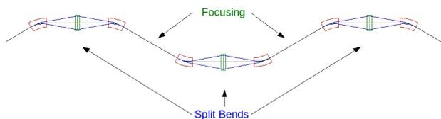
Figure 4: Chasman-Green DBA lattice for UH linear transport Diagnostic Chicane adaptation.
